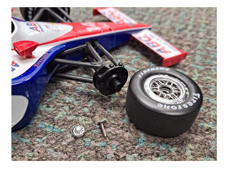
*#2 - Removing the front hubs (Optional)* Using an Xacto knife, cut off the melted plastic of the pegs located at the top and bottom of the front wheel hubs to remove them from the front suspension.
